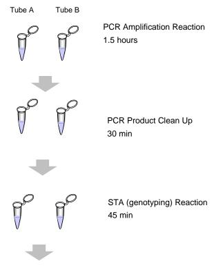
Capillary Electrophoresis Fragment Analysis 30-40 min
